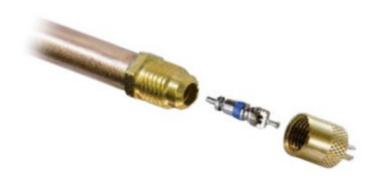
The 36LP Series comes with a CD2250 wrench cap and CD4460 valve core and is available in a variety of tube sizes ranging from 1/8" to 3/8". There are no pipe threads. Material is CDA 360 brass and standard refrigeration tubing. Tube length is approximately 2".
