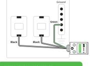
ALTERNATIVE WIRING METHOD: This SPD can be also be installed by splicing
