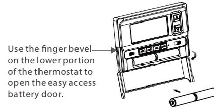
Use the finger bevel on the lower portion of the thermostat to open the easy access battery door.
